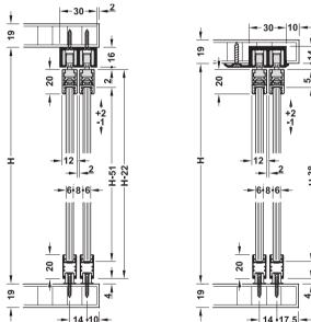
Clipo 16 GPPK; with glass fixing profile top and bottom
