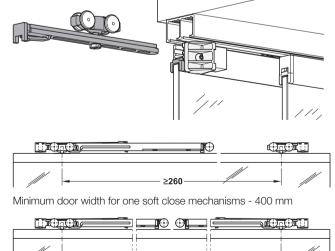
Minimum door width for two soft close mechanisms - 600 mm
