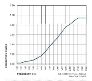
Composition has been engineered specifically to reduce and control reverberated (echo) noise in building interiors. Composition will also increase the sound transmission performance of walls. When adhered to one side of a wall, Composition provided a 3 STC point increase in the performance of the wall. For specific acoustic requirements, we recommend you consult an acoustic engineer.
